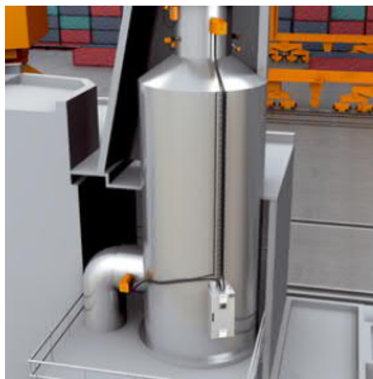
Measurement of SO x emission at scrubber inlet/outlet
